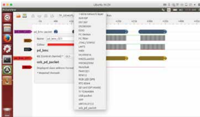
Capturing, displaying and decoding traces with the Sigrok tooling
