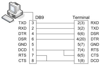
When using 2, 3, 5 only, loop-back each 7-8(4-5), 1-4-6(6-8-20). (numbers in parentheses are for DB25 connector.)
