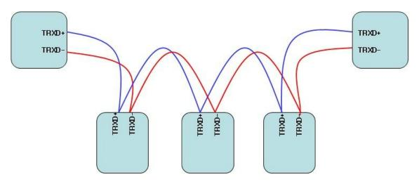
RS485, like LAN, uses Half Duplex Bus and has no classification between host and terminal.
