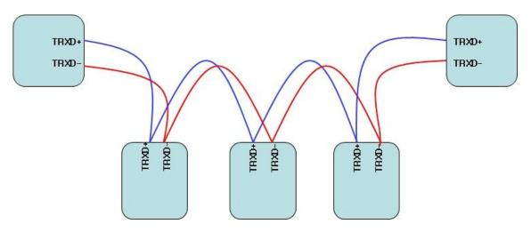
RS485, like LAN, uses Half Duplex Bus and has no classification between host and terminal.
