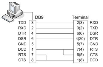
When using 2, 3, 5 only, loop-back each 7-8(4-5), 1-4-6(6-8-20). (numbers in parentheses are for DB25 connector.)
